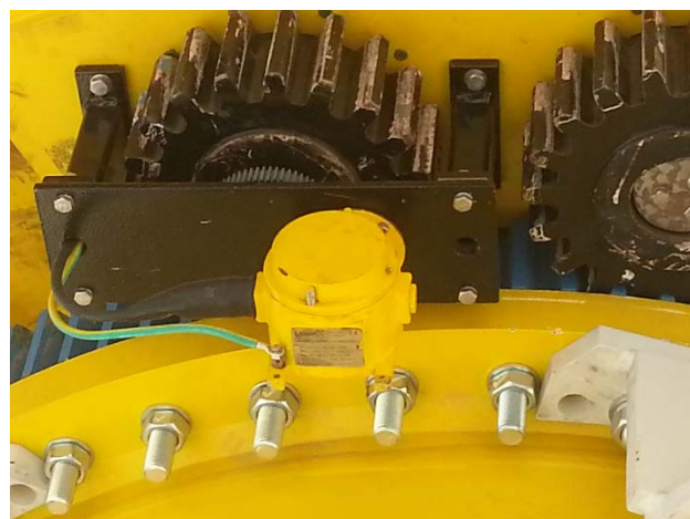
Rotation gear with limit switch
