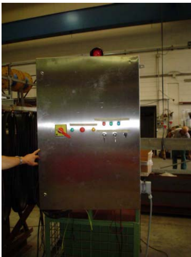
Control panel made of stainless steel AISI 316
