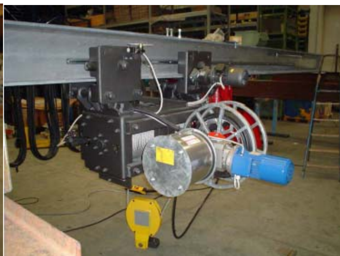
Electric operated cable reel for hoist feeding
