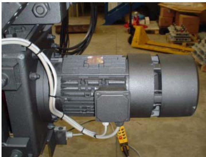
Lifting motor Bull, self-braking type with A/C brake
